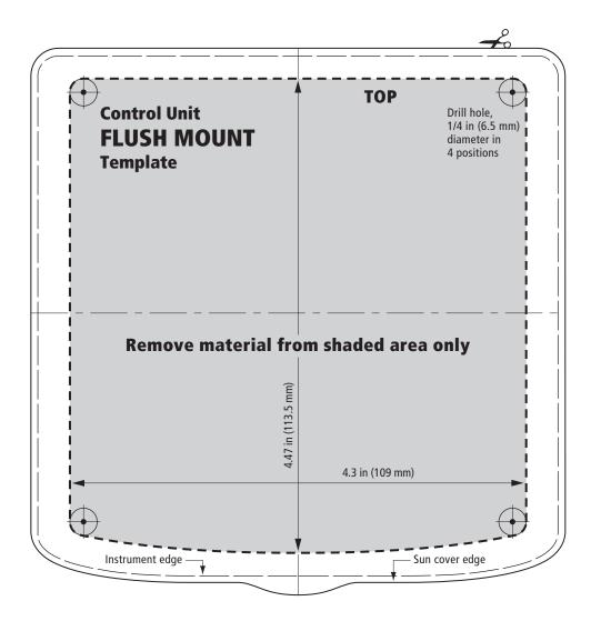
FLUSH MOUNT template for ST60+ Instruments
