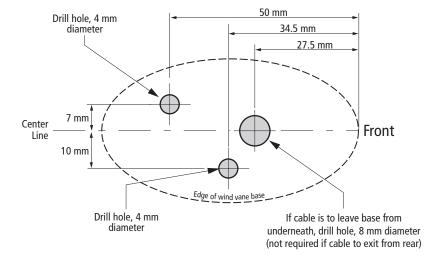
Wind vane drilling template
