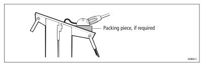
You can fit your wind vane so the cable leaves the wind vane base either from the rear (option A), or from underneath (option B).
