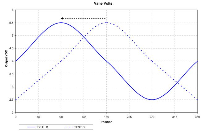
Note: Test Voltage indicates that vane transducer should be rotated 90° CCW
